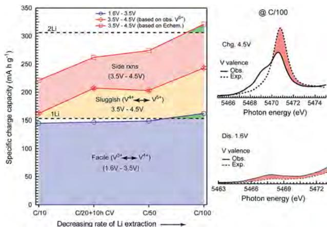
Fig. 5 Observed capacity and V valence during charge reveal facile V<sup>4+</sup>/V<sup>3+</sup> redox in the low-voltage region and sluggish V<sup>5+</sup>/V<sup>4+</sup> redox with pronounced side reactions contributions in the high-voltage region. This is shown by higher discrepancy between the observed (Obs.) and expected (Exp.) V valence for the sample charged to 4.5 V than for the sample discharged to 1.6 V at the slowest rate of C/100.
