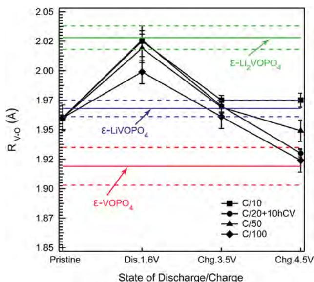
Fig. 4 Variation in the average V–O (metal–ligand) bond length of  $\epsilon$ -LiVOPO<sub>4</sub> samples electrochemically discharged/charged using different rates. The solid horizontal lines indicate the average V–O bond length of chemically prepared endmember phases and the dotted horizontal lines indicate the uncertainties of the fitted values.
