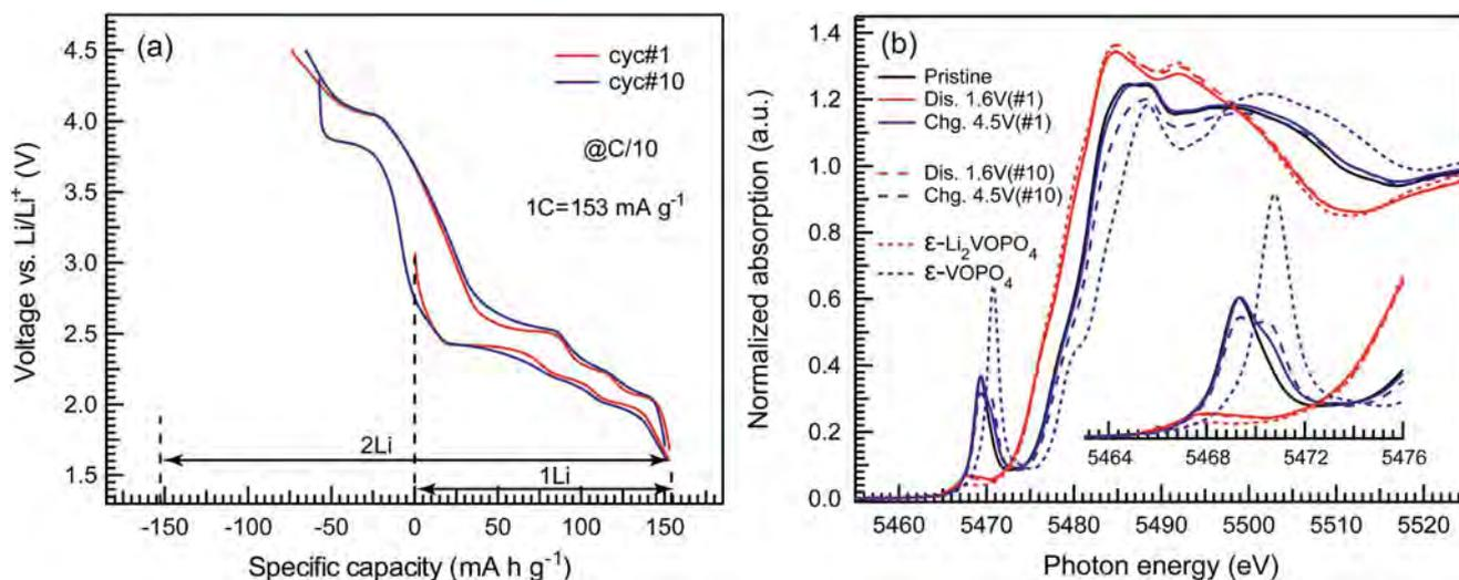
Fig. 6 (a) Voltage profiles and (b) the normalized V K-edge absorption spectra of ε-LiVOPO<sub>4</sub> samples discharged to 1.6 V and charged to 4.5 V in the 1st and 10th cycles.
