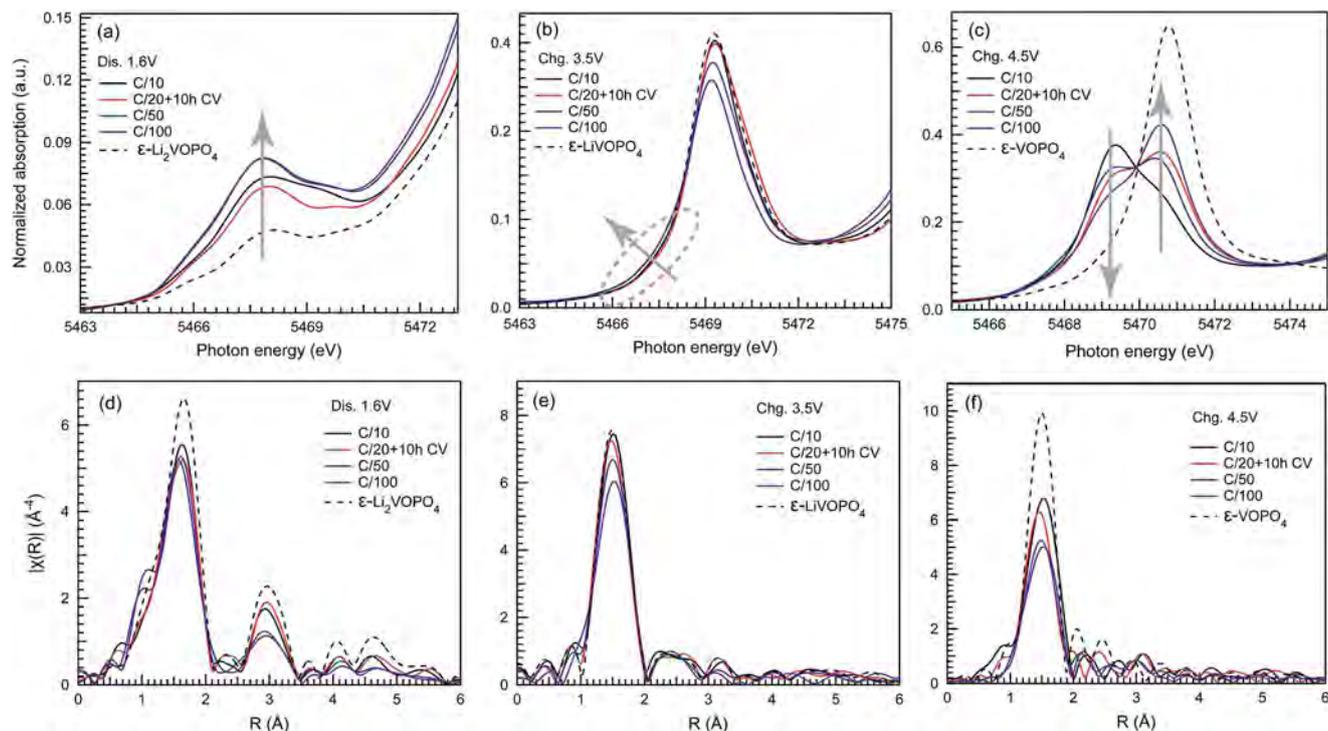
Fig. 3 Comparison of the pre-edge regions (top) and EXAFS signals (bottom) of  $\epsilon$ -LiVOPO<sub>4</sub> samples discharged to 1.6 V (a and d), charged to 3.5 V (b and e) and charged to 4.5 V (c and f) using different rates.
