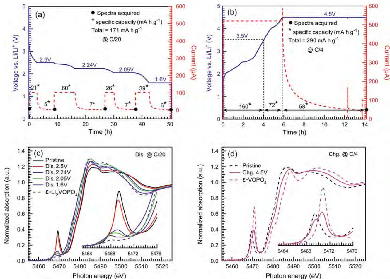
Fig. 2 Variation in the cell voltage and current during operando XAS measurements upon (a) discharge to 1.6 V at C/20 and (b) subsequent charge to 4.5 V at C/4. The normalized V K-edge absorption spectra of  $\epsilon$ -LiVOPO<sub>4</sub> for various states of discharge and charge are presented in (c) and (d), respectively, with the inset showing an enlarged pre-edge region of these spectra.
