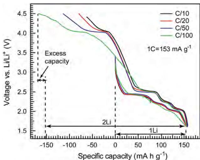
Fig. 1 Voltage profiles of  $\epsilon$ -LiVOPO<sub>4</sub> during first discharge to 1.6 V and subsequent charge to 4.5 V using different rates.
